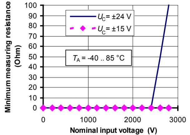
Figure 2: Minimum measuring resistance.
