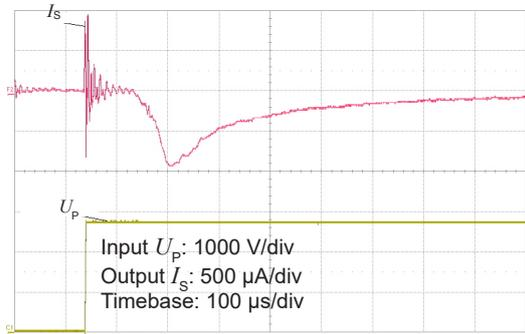
Figure 13: Typical common mode perturbation (2800 V step with 6 kV/µs  $R_M = 100 \Omega$ )
