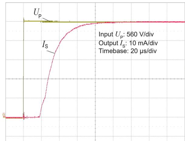
Figure 6: Typical step response (0 to 2800 V)
