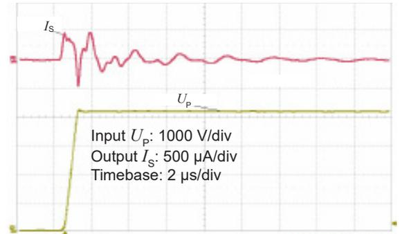
Figure 14: Detail of typical common mode perturbation (2800 V step with 6 kV/µs,  $R_M = 100 \Omega$ )
